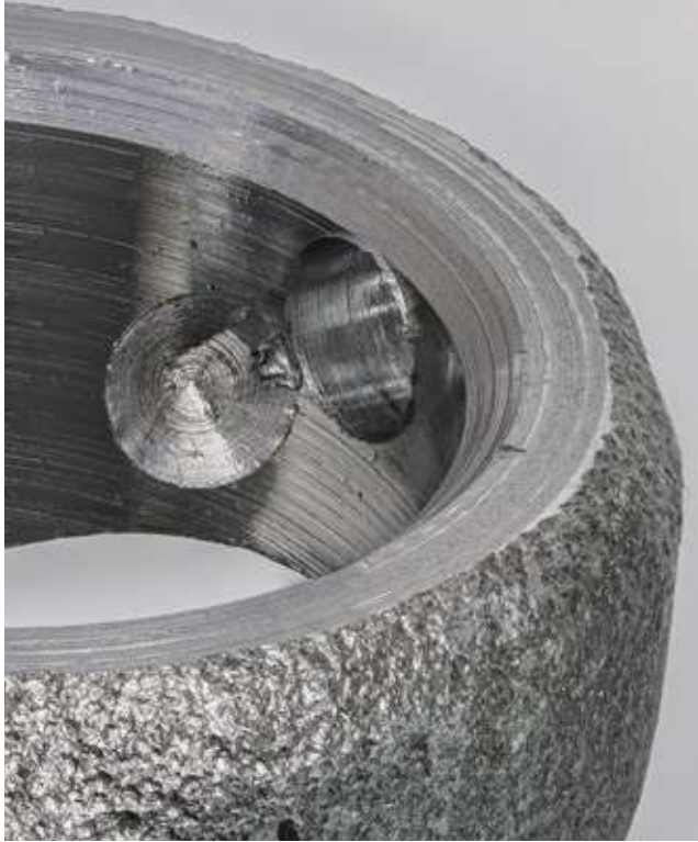
Part of a piston rod made of C70 steel. When using a standard drill (left), a relatively large burr is created on the curved surface at the exit of the Bore and a cap remains. When using the ExBurrDrill (right), only a minimal burr can be seen at the exit edge of the bore, a cap is not created.
