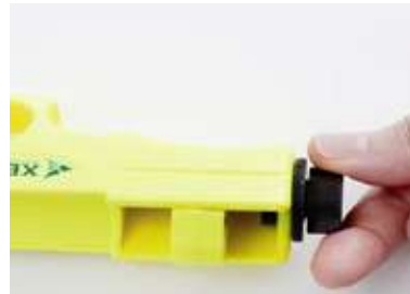
1. Move the brush rest using adjustment knob to set the amount of brush projection.
