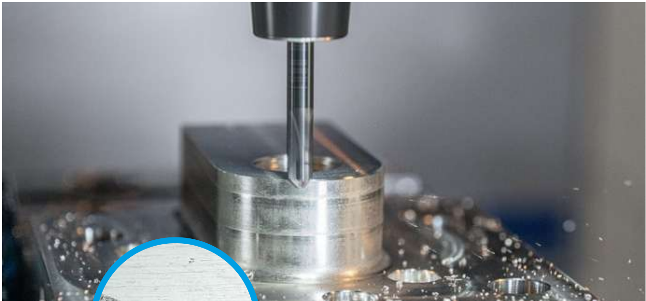
Picture above: Here you can clearly see the burr (left of the cutter) and the already deburred contour (right of the cutter).
