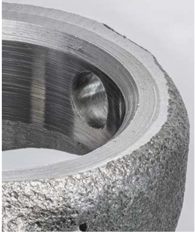
Part of a piston rod made of C70 steel. When using a standard drill (left), a relatively large burr is created on the curved surface at the exit of the Bore and a cap remains. When using the ExBurrDrill (right), only a minimal burr can be seen at the exit edge of the bore, a cap is not created.
