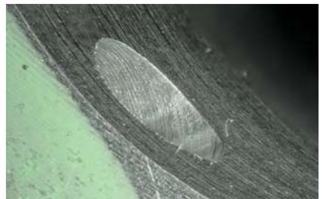
Bore exit after using the ExBurrDrill in aluminum
