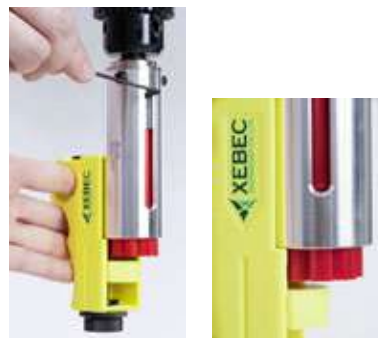
3. Loosen the locking screw of the brush. Hold the unit in one hand and align the sleeve rest with sleeve tip.
