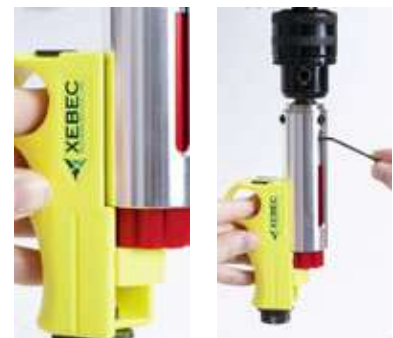
4. Tighten the locking screws to secure brush in place.
