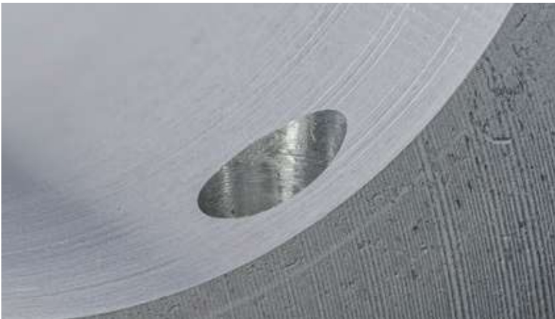
ABOVE: Off-axis bore exit into the cross bore in an aluminum component. With the ExBurrDrill, almost no burr can be measured even with this type of machining.
