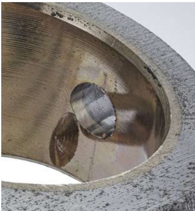
Piston rod bearing with bore entry in C70 steel and bore exit (bearing bush) made of CuZn31Si1. On the left a standard drill was used, on the right the KEMPF ExBurrDrill. The differences are significant.
