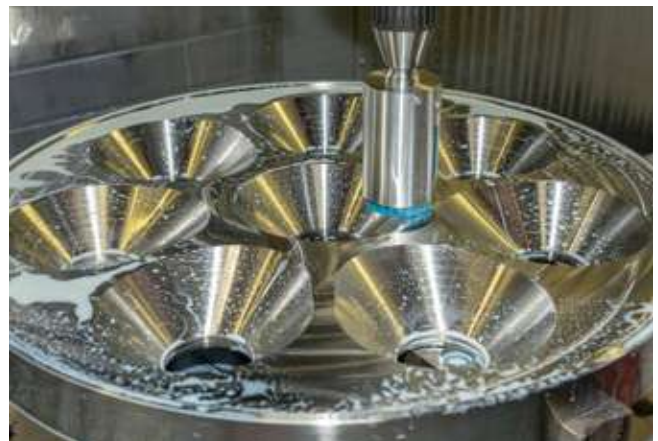
Picture below right: The surface and edges of a steel closure for pressure vessels are polished and deburred after milling with the ceramic fiber brush.
